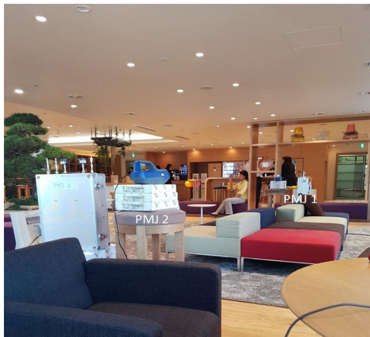
Figure 6. Picture of the PMJ coffee corner. The instruments used for air quality measurements are located on both sides of the room (PMJ 1, PMJ 2) [59].
