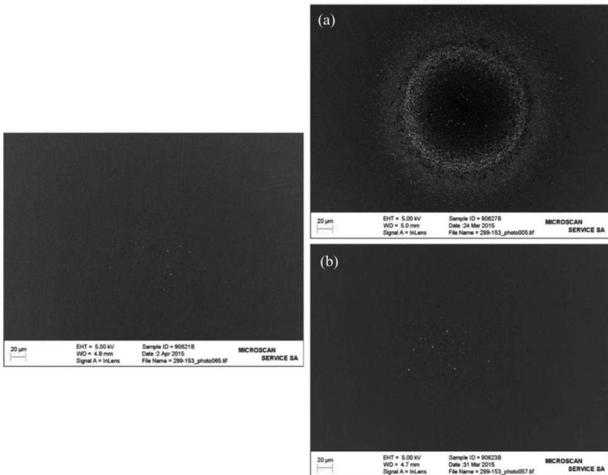
Figure 11. Pictures showing accumulated submicron particles from (a) mainstream 3R4F smoke and (b) EHTS aerosol. The picture on the left side is the related blank prior to the start of aerosol collection [90].
