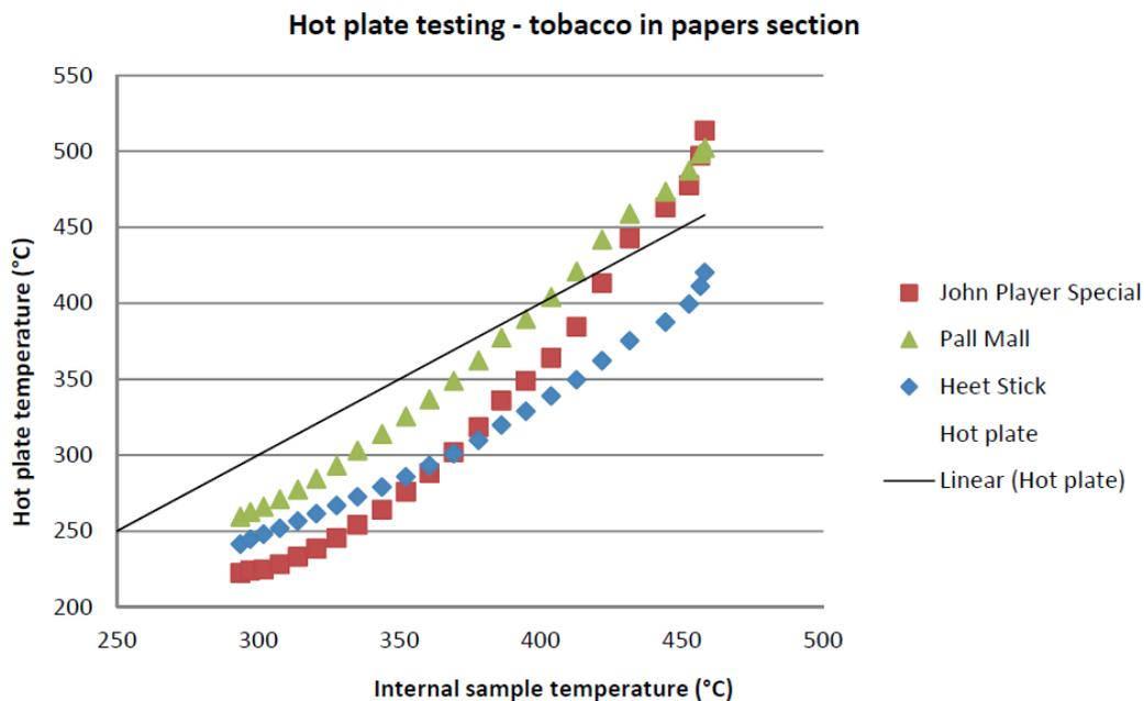
Figure 7. Hot plate auto ignition testing [74]. Heet Stick in the legend refers to the EHTP.
