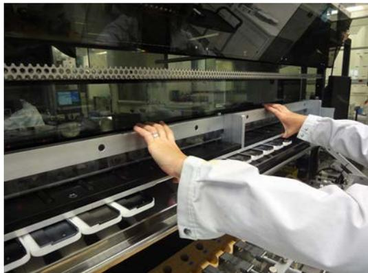
If the activation bar is not used, devices can be activated manually. Activate the THD by pressing the central start switch gently for 4 seconds. The LED will flash for 20 seconds indicating that the pre-heating phase has started. Once the pre-heating is complete, the LED will stop flashing. **Wait the end of the pre-heating phase** before starting the aerosol generation cycle.
