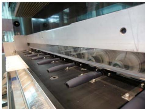
11. Activate the THDs by pressing gently the top of the activation bar for 4 seconds. The LEDs on the THDs will flash for 20 seconds indicating that the pre-heating phase has started. Once the pre-heating is completed, the LEDs will stop flashing. **Wait the end of the pre-heating phase** before starting the aerosol generation cycle.
