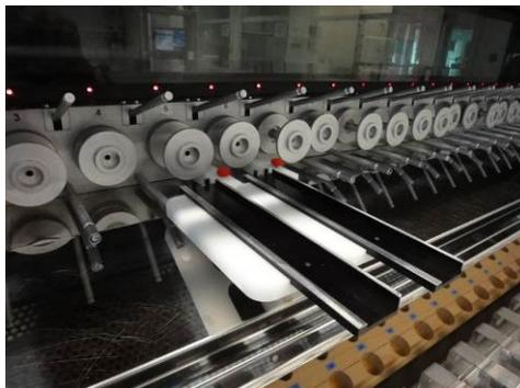
4. Install the adaptor bracket of the activation bar with its plate from the position 1 to 20. Except at position 5-7 and 14-16 to allow the activation of the bar by the operator (refer to picture in step 11)
