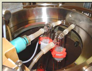
Fig. 3: The 20-port rotary smoking machine (left) and the two wash bottles connected in series (right)
