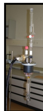
The bubbler with the trapping solution on the top of the trap (should be inside the instrument)
