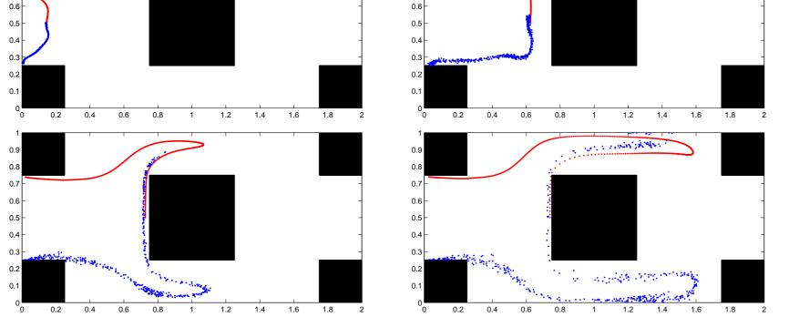
• Snapshots of particle positions. Initially particles are placed on x = 0, z = 0 line. Brownian force is applied on blue particles, while red particles move only due to the Stokes drag.
