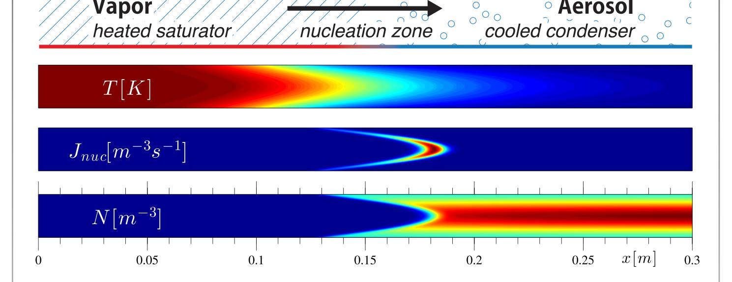
The droplet number concentration depends on the temperature of the saturator,  $T_{sat}$ . We find a reasonable agreement between experiment and simulation:
