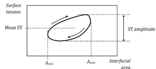
Figure 1. Definition of the mean ST and the ST amplitude in the experimental relationship (hysteresis loop).
