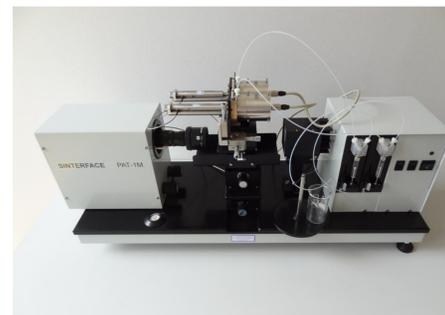
Figure 3. PAT-1M tensiometer (picture adopted from www.sinterface.com).
