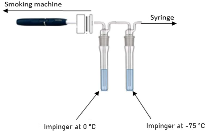
Aerosol collection using 2 impingers containing each 10 mL of a mixture of ethyl acetate / MeOH (95%/5%) cooled at 0°C and -75°C
