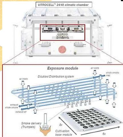
A climatic chamber with an exposure module
