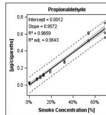
Whole-smoke application (multi-dilution) and quantification of nicotine and 8 different carbonyls inside the VITROCELL® 24/48 exposure chamber over a concentration range of 7–69% cigarette smoke.
