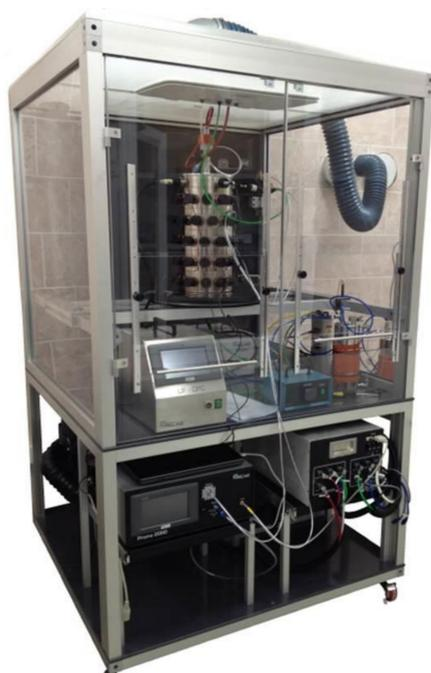
Figure 1: Snapshot of a NOEC produced by CH Technologies (USA) and assembled with measurement equipment (Palas) inside a laboratory enclosure.
