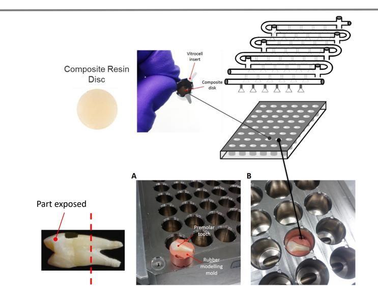
Composite resins and premolar teeth were allocated in the Vitrocell<sup>®</sup> 24/48 exposure plate
