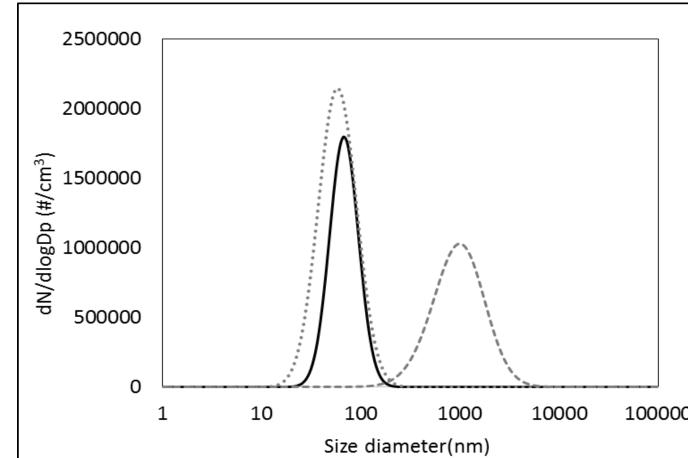
**Figure 4**: Coating removal experiments. The black lognormal-fitted curve corresponds to the measured size distribution of NaCI seeds (at 30°C). The dashed and the dotted lognormal-fitted curves represent the size distribution of glycerin-coated NaCl particles after they passage in the thermo-denuder when the temperature was set at 30 and 300°C, respectively
