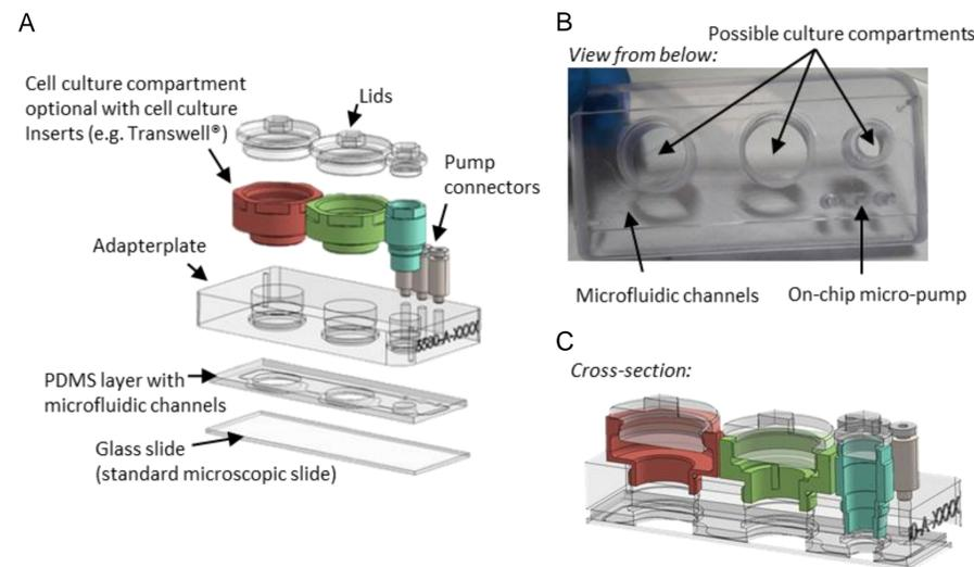
**Figure 1: The Multi-Organ-Chip (MOC) platform and the experimental procedure for the chip culture at a glance.** (A) Components of the 3-Organ-Chip optimized for medium supply (3-OCplus). (B) Bottom view of the 3-OCplus. (C) Cross-section of the 3-OCplus.
