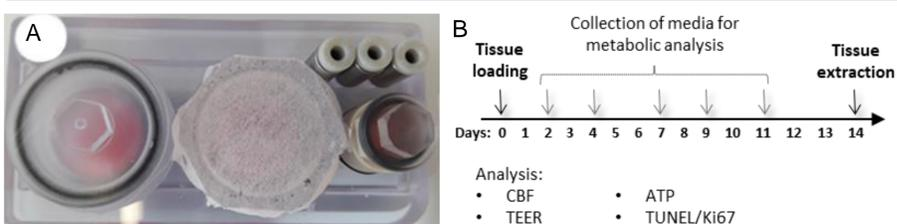
**Figure 2: Experimental set-up and Timeline of chip experiment.** (A) Illustration of the 3-OCplus with breathable lid above the lung culture compartment. (B) Timeline of the 14-day experiment. Medium is exchanged every 2<sup>nd</sup> to 3<sup>rd</sup> day.
