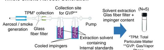
Figure 1. <sup>a</sup>Whole smoke aerosol generation using pad + impinger and <sup>b</sup>Cold Trap aerosol generation by means of a cold trap system maintained at  $-196^{\circ}\text{C}$  ( $-320^{\circ}\text{F}$ )
