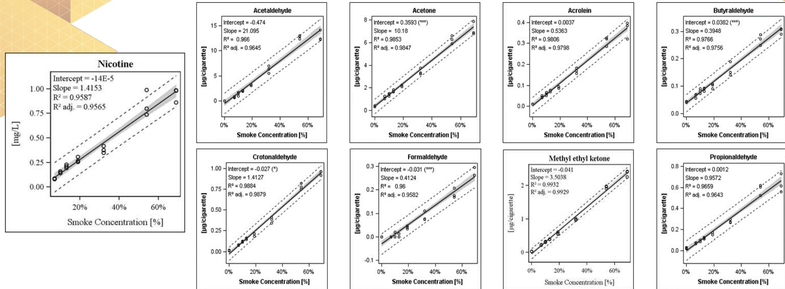
Whole-smoke application (multi-dilution) and quantification of nicotine and 8 different carbonyls inside the VITROCELL® 24/48 exposure chamber over a concentration range of 7–69% cigarette smoke.
