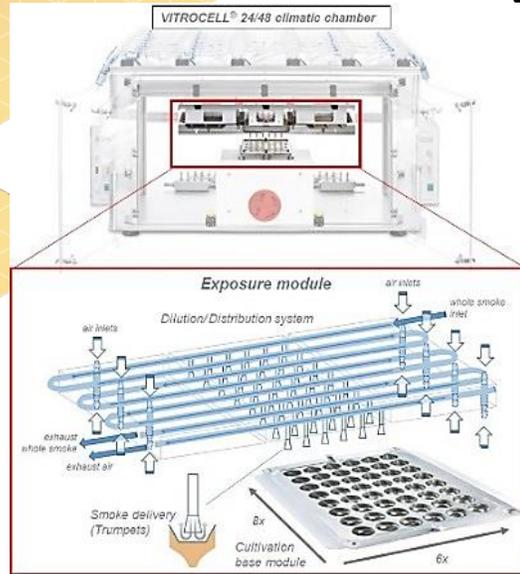
A climatic chamber with an exposure module
