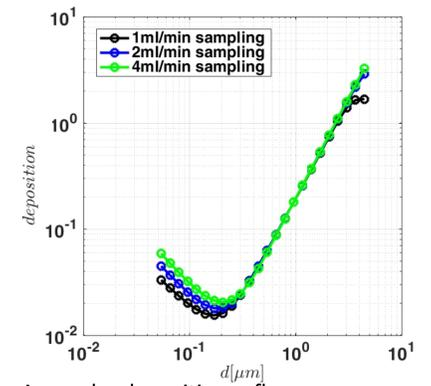
Aerosol deposition flux versus particle diameter for three sampling flow rates (1ml/min; 2ml/min; 4ml/min). Deposition for larger particles is dominated by gravity and independent of the low sampling rate.
