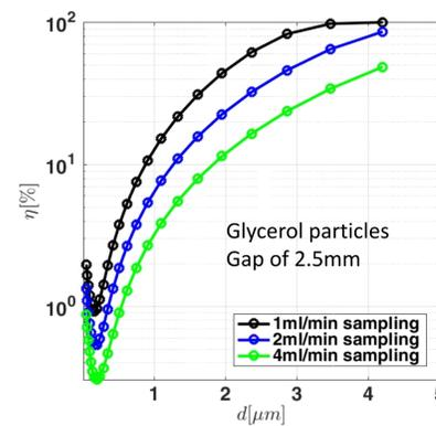
Aerosol deposition efficiency versus particle diameter for the three sampling flow rates. Efficiency decreases with increasing flow rate. Full deposition can be reached for large particles and low sampling rates.
