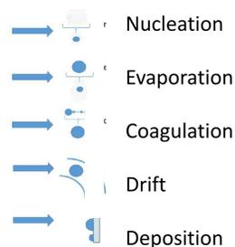
The aerosol is modeled within an Eulerian-Eulerian framework with the aerosol size distribution and aerosol dynamics represented by either a sectional or a two-moment method.
