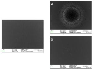
Figure 2: pictures showing accumulated submicron particles from the thermo-denuder treated mainstream of a) 3R4F smoke and b) THS2.2 aerosol. The picture on the left side is the related blank prior aerosol collection started. *We would like to thank Microscan Service SA (Rue de la Blancherie 17, 1022 Chavannes-près-Renens, Suisse) to have performed the SEM/EDX analyses, provided* scientific expertise and SEM pictures
