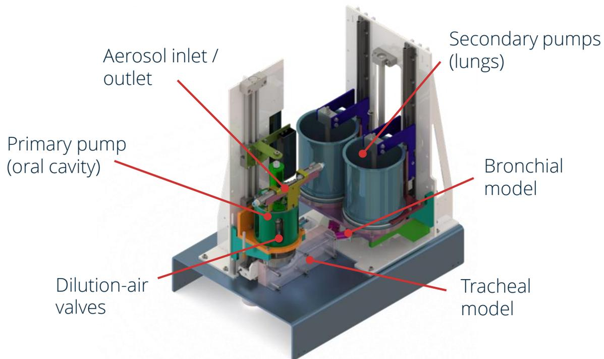
An array of piston pumps connected by a model of the conducting airways
