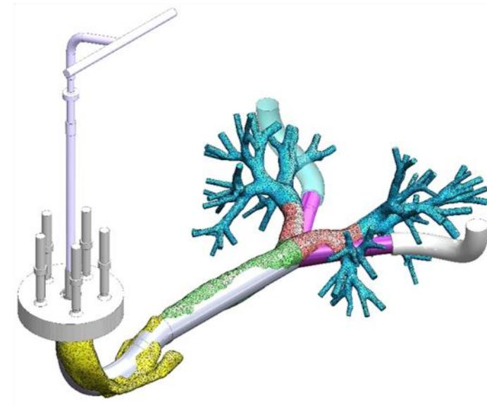
Dimensions and shape of the airways are based on *in vivo* data\*, in the prototype version of the system only realized to G1 (main bronchi)
