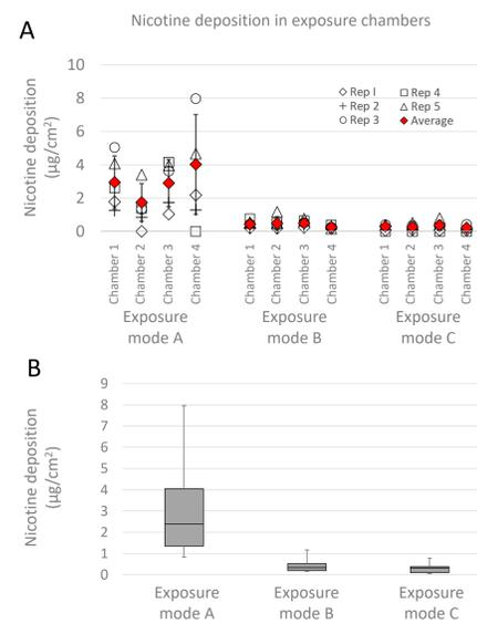
Figure 3: Nicotine deposition in the exposure chambers. A) resolved by experimental repetition and exposure chamber, B) global across the four exposure chambers and five experimental repetitions. Error bars in A) indicate standard deviations, error bars in B) indicate the lowest and the highest measured values.
