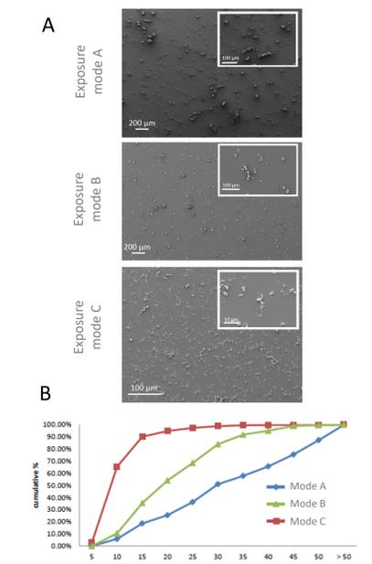
Figure 4: A) SE micrographs of particles deposited under the three exposure modes. B) cumulative particle size distribution measured in the SE micrographs.
