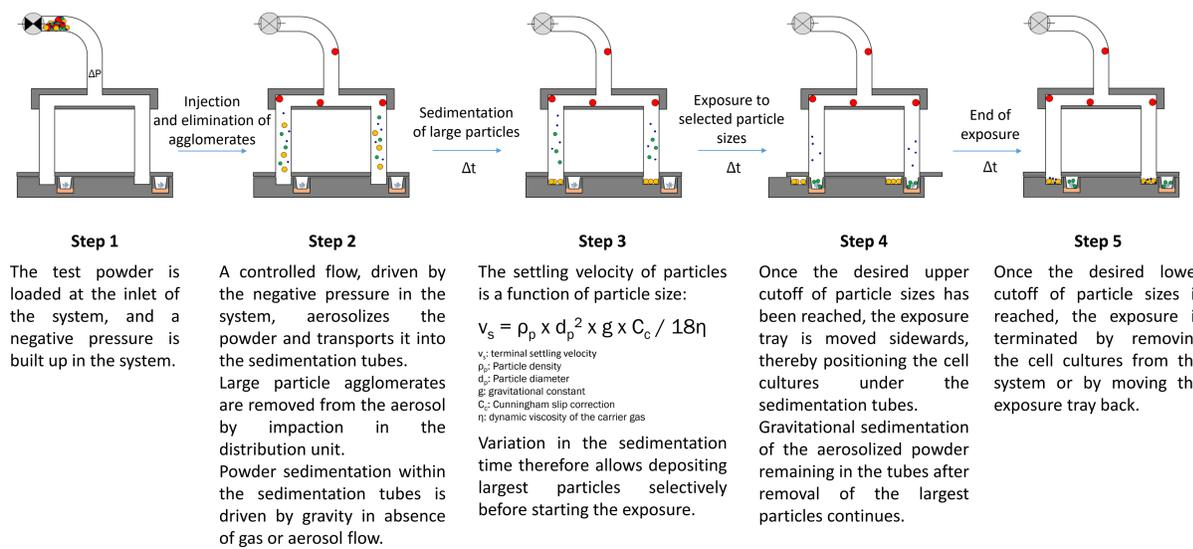
Figure 1: Overview of the Vitrocell® Powder Chamber and the system's working principle.
