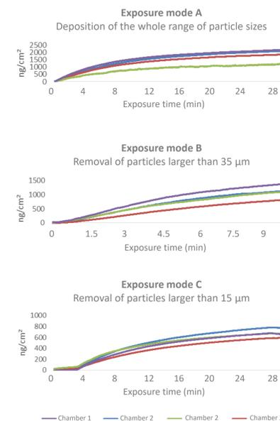
Figure 2: Real-time powder mass deposition during the exposures. The figure shows one representative repetition for each tested exposure mode.
