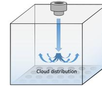
2) Due to its kinetic energy and convection, the aerosol distributes inside the chamber
