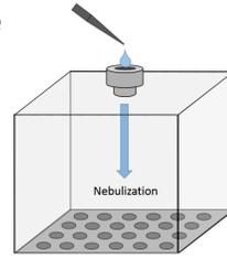
1) The test liquid is nebulized into the aerosol chamber
