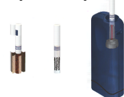
explosion view showing cigarette construction consumed cigarette showing burn marks cigarette in lighter, ready for use
