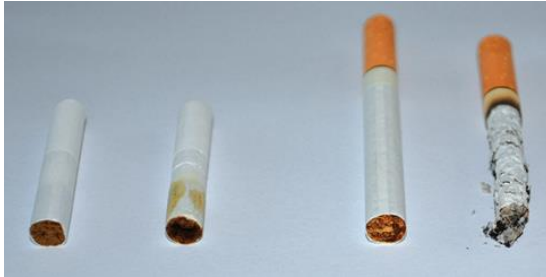
Figure 2: Comparison of unused and used THS Tobacco Stick (left) and conventional cigarettes (right). The structural integrity of the Tobacco Stick is retained after use and no ash is formed (left pictures), in contrast to a cigarette (right pictures).
