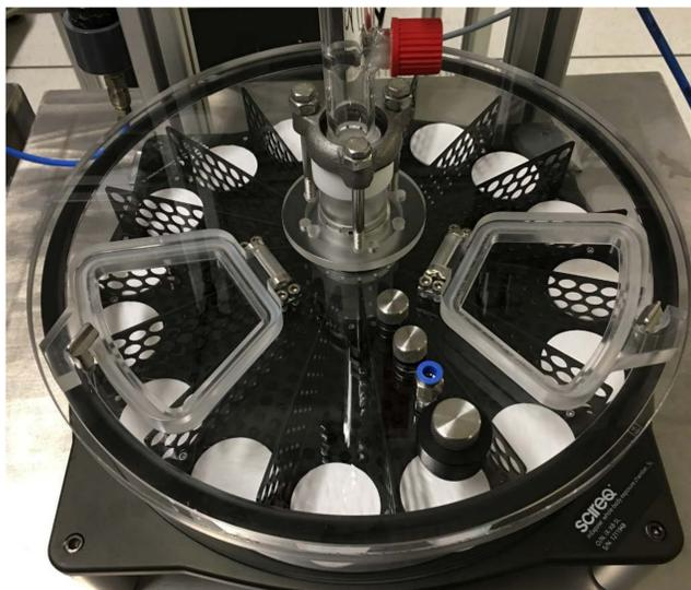
**Figure 4.** Positioning of filter pads in the sWBEC for determining the spatial homogeneity of aerosol concentration.
