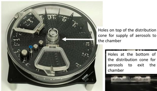
Holes on top of the distribution cone for supply of aerosols to the chamber
