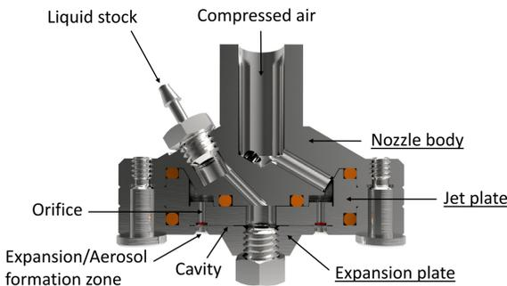
**Figure 2.** BLAM, vertical cross-sectional view.
