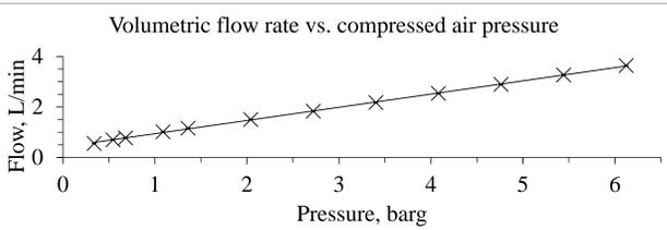
**Figure 3.** Single-orifice BLAM flow rate vs. compressed air pressure.
