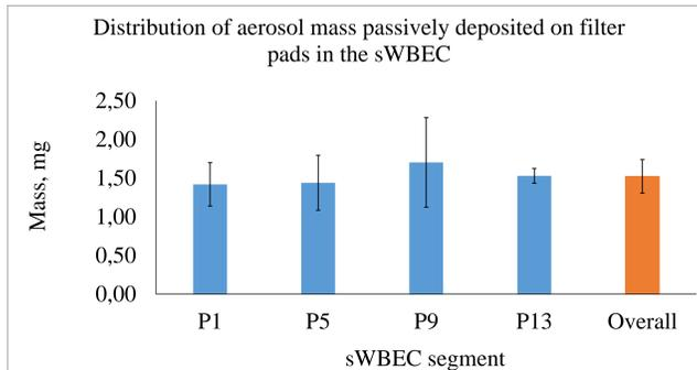
**Figure 5.** Aerosol mass deposited at different positions in the sWBEC over 60 minutes.
