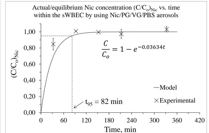
**Figure 7.** Nicotine concentration profile in the sWBEC, showing  $t_{95} = 82$  min.
