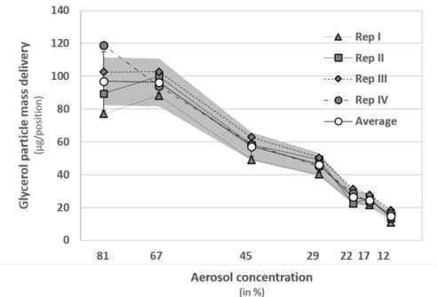
Figure 4: Aerosol mass delivery as function of aerosol dilution. Individual exposure runs and the average over four repeated exposures are shown. Error bars represent standard deviations between the four runs. The grey area indicates the average ± 15%.
