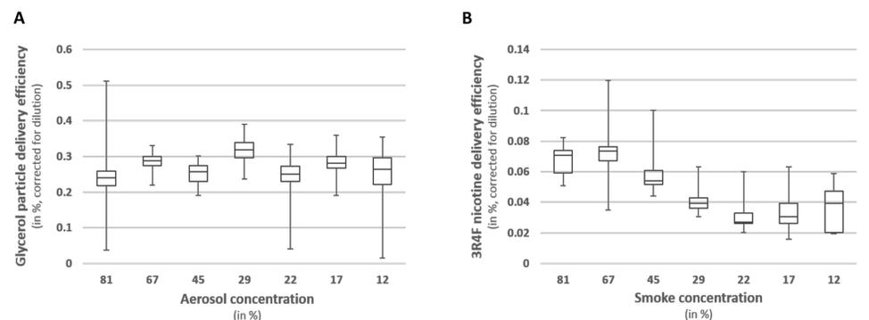
Figure 6: Dilution corrected delivery efficiency of A) glycerol aerosol and B) 3R4F smoke. Delivery efficiencies were calculated according to Eq 2, the boxplots represent first, second and third quartile, minimal and maximal value.
