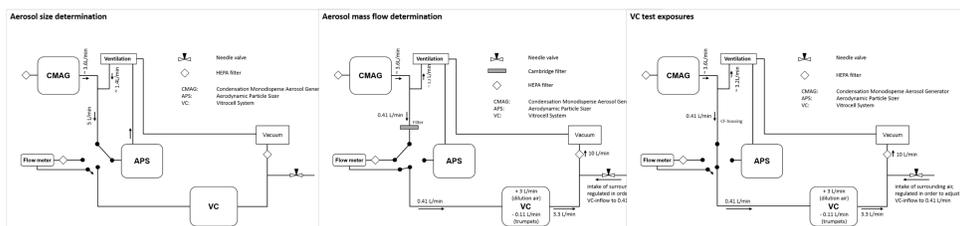
Figure 3: Physical setup of the instrumentation used for aerosol characterization and test exposures
