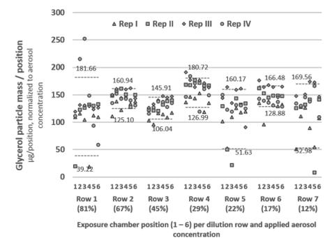
Figure 5: Aerosol mass delivery per exposure chamber, normalized to the applied aerosol concentration. Dashed lines and numbers indicate the 10<sup>th</sup> and 90<sup>th</sup> percentiles.
