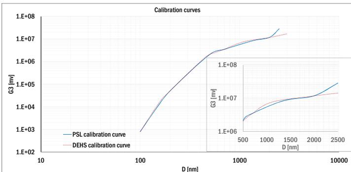
Figure 1: Calibration curves for two aerosol materials.
