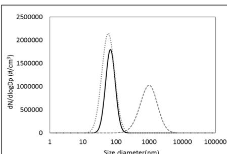
Figure 4: Coating removal experiments. The black lognormal-fitted curve corresponds to the measured size distribution of NaCl seeds (at 30°C). The dashed and the dotted lognormal-fitted curves represent the size distribution of glycerin-coated NaCl particles after they passage in the thermo-denuder when the temperature was set at 30 and 300°C, respectively
