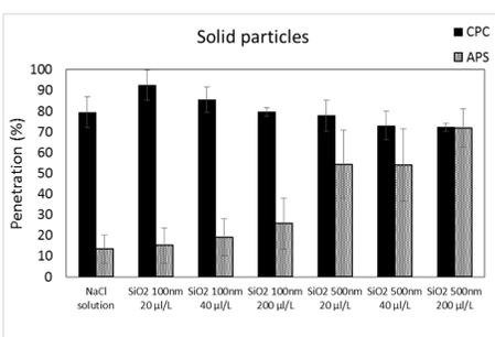
Figure 2: Aerosol penetration for SiO<sub>2</sub> and NaCl particles using CPC and APS instruments
