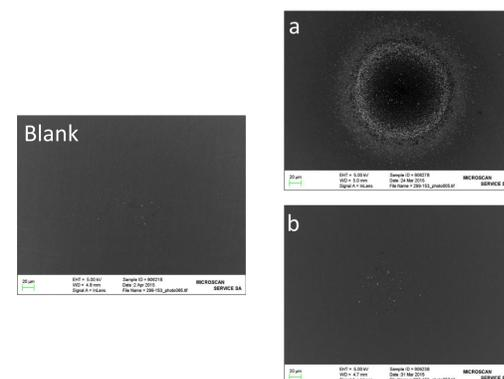
Figure 6: Pictures showing accumulated submicron particles from the thermo-denuder treated mainstream of a) 3R4F smoke and b) THS 2.2 aerosol. SEM/EDX analyses were performed by Microscan Service SA (Rue de la Blancherie 17, 1022 Chavannes-près-Renens, Suisse)
